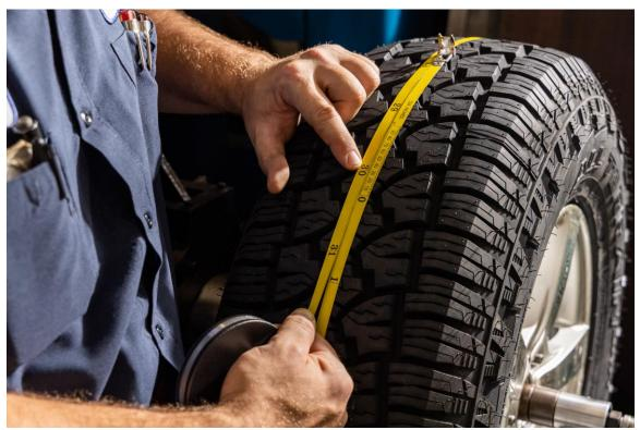
Photograph A5.5: Measuring Outside Diameter
