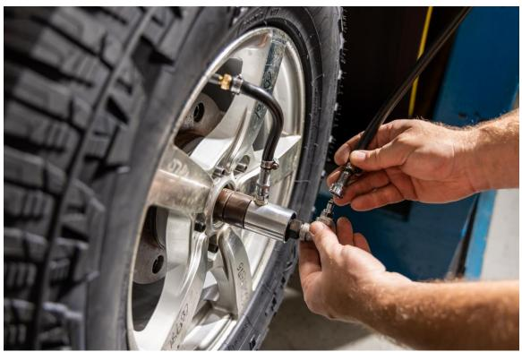
Photograph A5.2: Connecting Tire to Air Pressure
