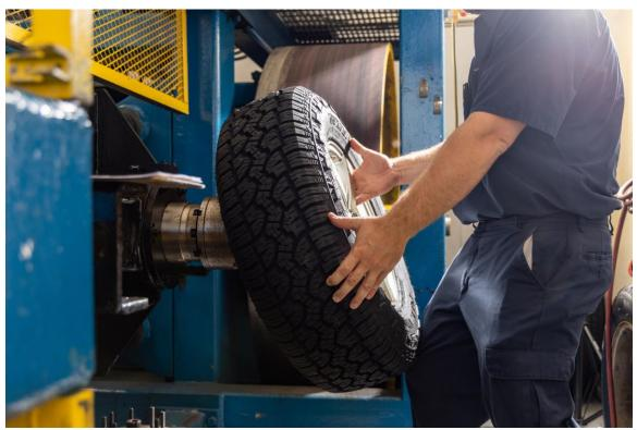
Photograph A5.1: Mounting Rolling Resistance Tire
