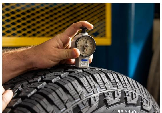
Photograph A5.3: Measuring Tread Hardness
